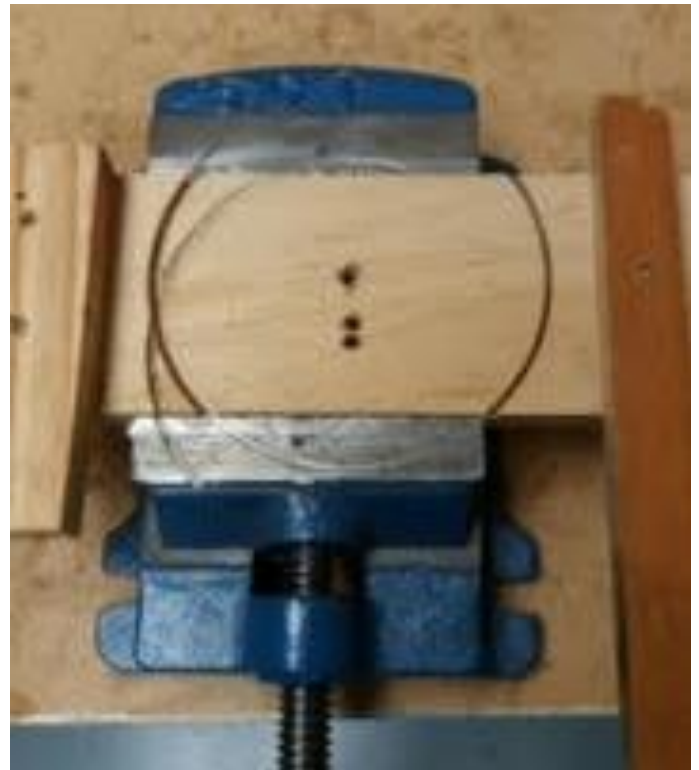
Vice recently damaged by incorrect use
